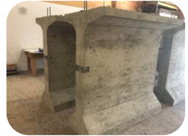
Above: New bridge girder sections ready to be used for Anatomy of a Bridge classes at NPS.
